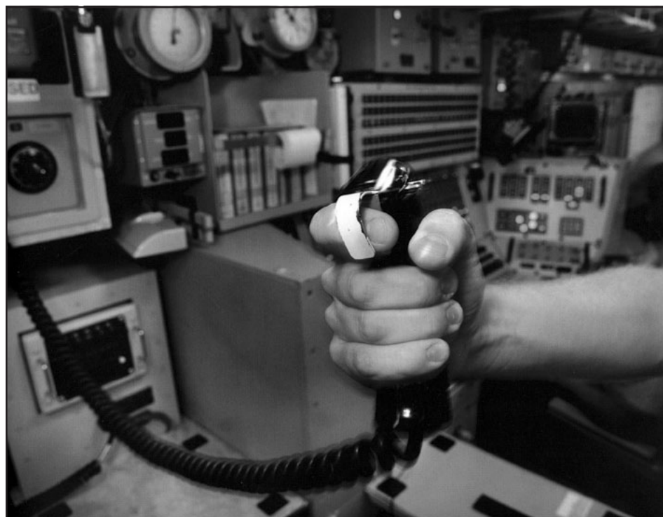
The launch trigger for a Trident missile. Photo by Paul Shambroom, from his book, Face to Face with the Bomb: Nuclear Reality after the Cold War.
