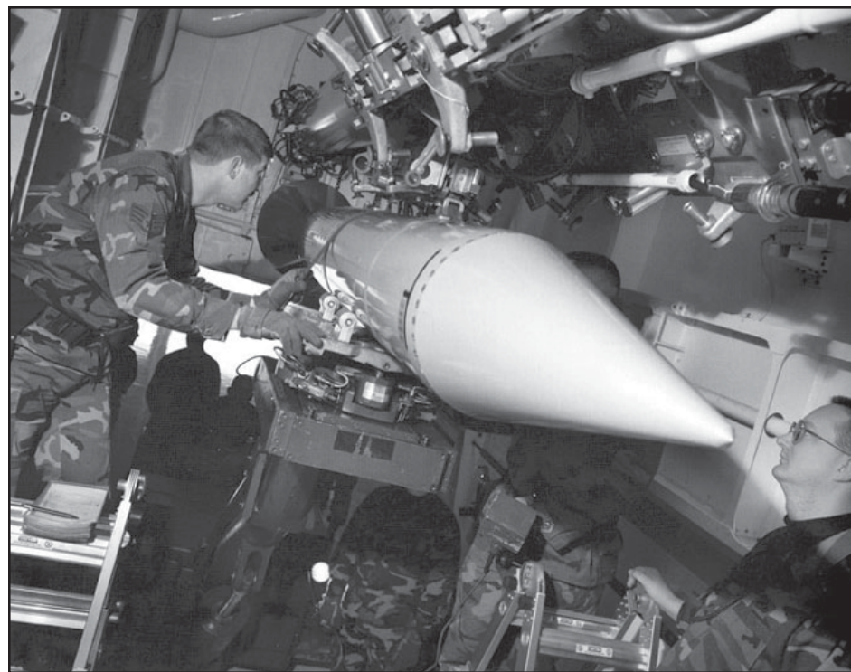
A B61-11 earth-penetrating bomb in the bomb bay of a B-2 Bomber. Photo by Paul Shambroom, from his recent book, Face to Face with the Bomb: Nuclear Reality after the Cold War.
